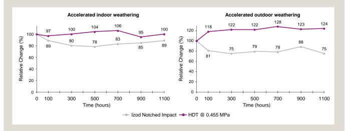
Note: For the indoor method, it is possible to infer that accelerated weathering times of 400 and 800 hours correspond to ca. 5 and 10 years of ageing in normal conditions, respectively. For the outdoor method, it is possible to infer that accelerated weathering times of 400 and 800 hours correspond to ca. 8 and 16 months of ageing in normal conditions, respectively.
